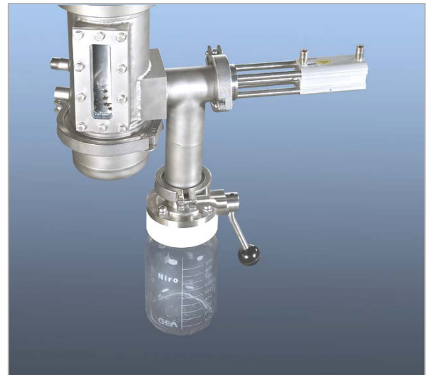
Continuous powder collection under the fluid bed
