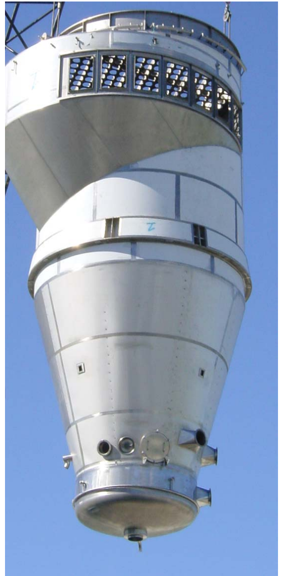
Bag filter housing with exhaust air inlet and bottom fluidization.
