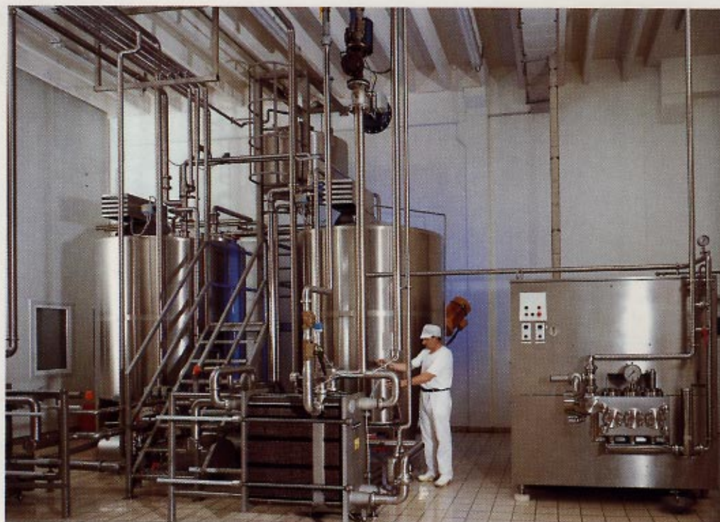
Mixing tanks – pasteurizer – homogenizer
