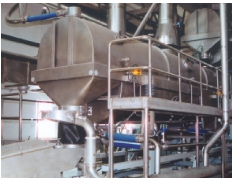
Vibro-Fluidizers® for powder after treatment: drying and cooling.
