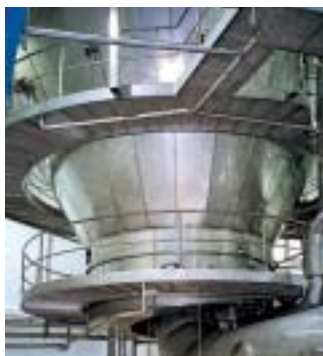
Conical part of spray drying chamber with the integrated fluid bed in a CDI Dryer
