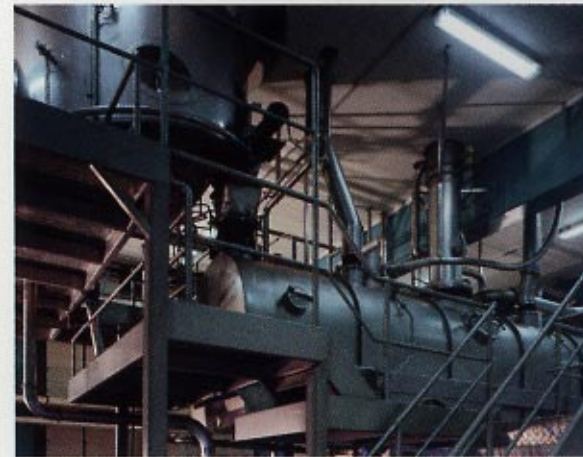
CIP nozzles installed to clean the integrated fluid bed of the spray dryer and the attached vibrating fluid bed (VIBRO-FLUIDIZER®).
