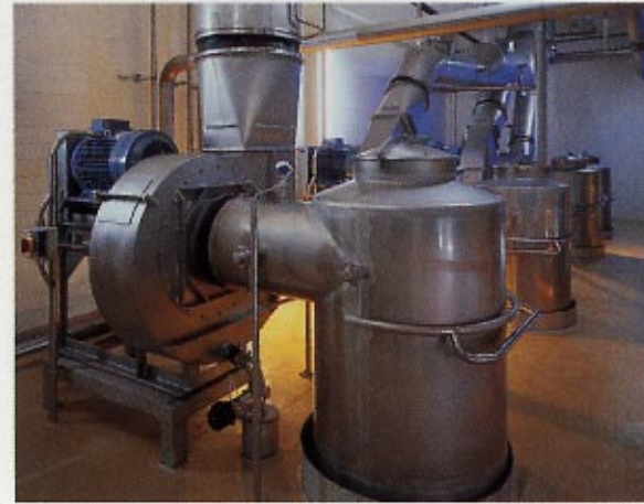
High efficiency cyclones equipped with CIP nozzles mounted in the top and around the main body.
