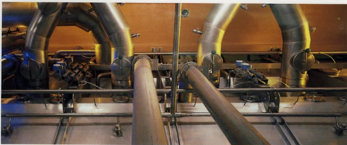
Top view of the horizontal section of the FILTERMAT® spray dryer with side-mounted CIP nozzles.
