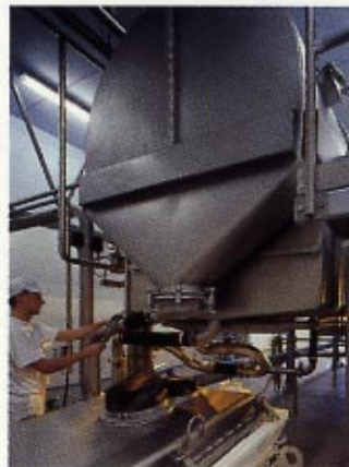
Preparing the VIBRO-FLUIDIZER® for CIP cleaning by placing, at the powder outlet, a funnel which returns the cleaning liquid to the CIP kitchen.
