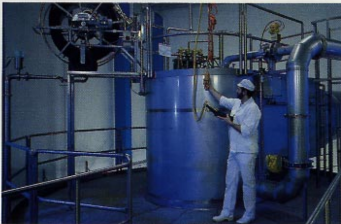
Preparing the VIBRO-FLUIDIZER® for CIP cleaning by placing, at the powder outlet, a funnel which returns the cleaning liquid to the CIP kitchen.
