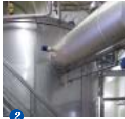
2 Spray dryer - side view
