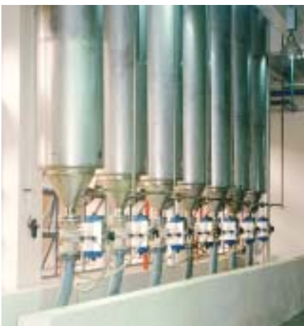
Conventional batch percolator – bottom view
