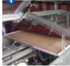
4 Freeze drying: Tray going into the CONRAD™ freeze dryer
