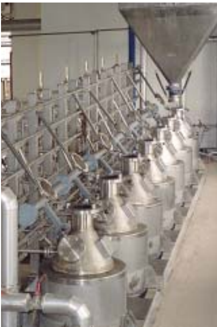
Conventional batch percolator – top view
