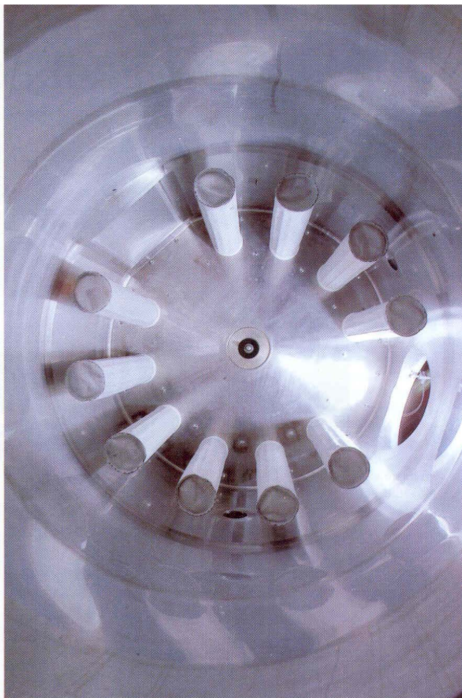
Figure 3: Bag filters integrated in spray drying chambers.
